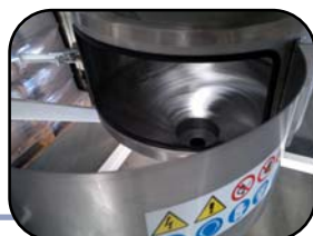
INSPECTION HOOD DETAIL
